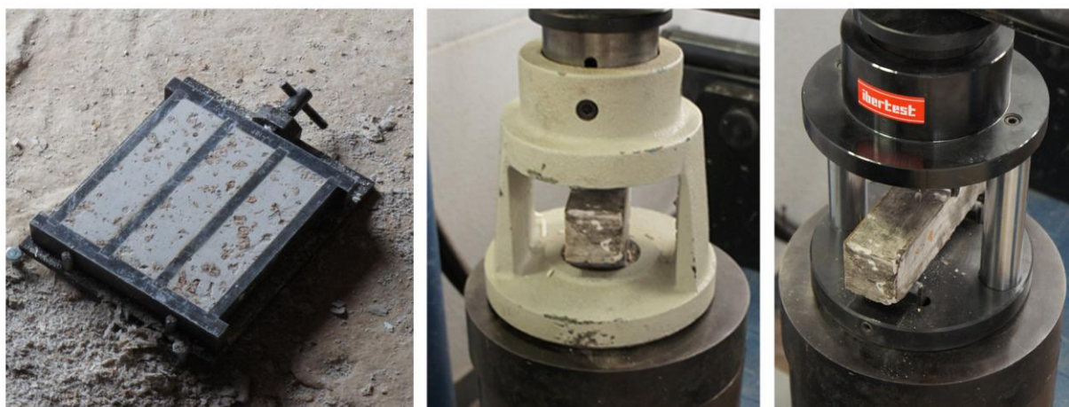
Figure 7. Mechanical tests for fibre-bonding interface (Cristini/Ruiz-Checa)
