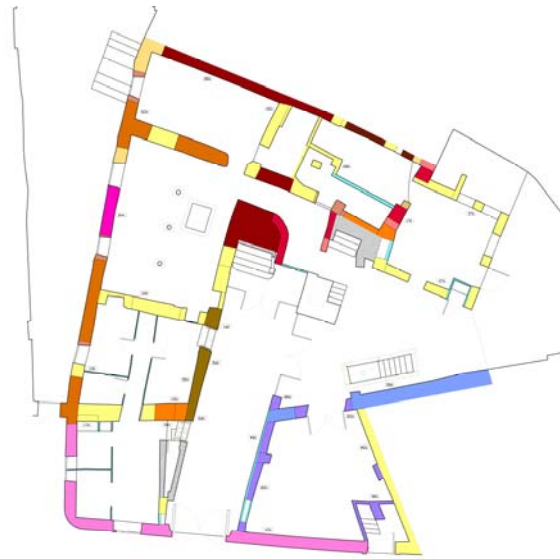
Figure 4. Marqués de Caro Palace. Layout of the ground floor with the type of fabrics found shown in different colours
