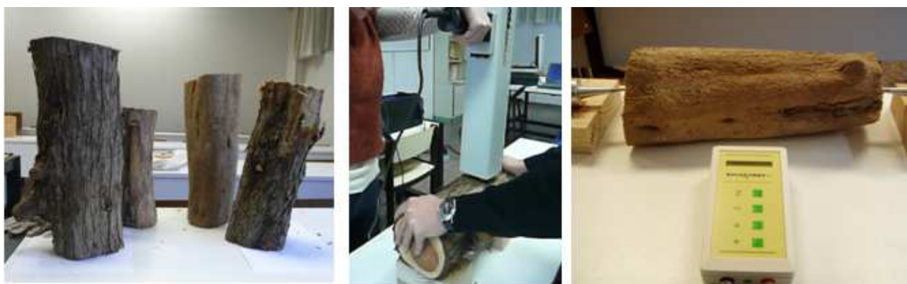
Fig.3 (from the left) Juniper timber samples: resistograph test and ultrasound system test (RUIZ CRISTINI)
