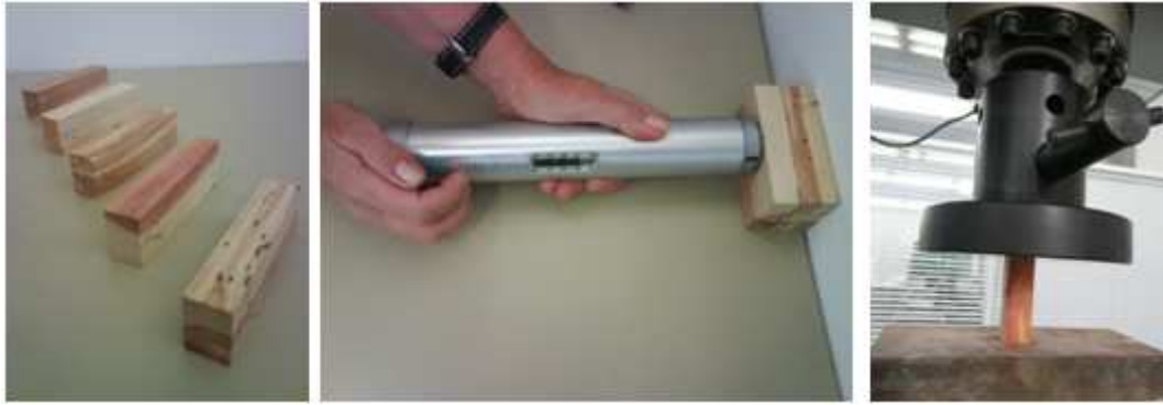
Fig.4 (from the left) Juniper timber normalized samples: Pylodin test and endurance resistance test (RUIZ CRISTINI)
